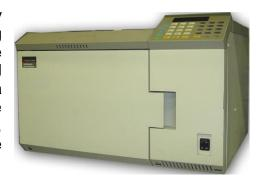
Carrier gas: nitrogenDetector: FID, ECD
